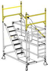
7 Sitting on the platform remove the guardrails (e.g. the reverse of steps 4 - 5).
