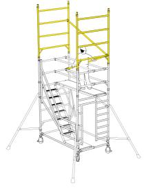
Standing on the fully guardrailed platform, fit the stairway guard rail to the front of the tower. The lower claws fit above and below the cross members of the 2 rung (1.0m) span frame, as shown. Fit the next stair case above the first with the landing claws fitted to the top cross member of the walk through frame.
