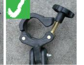
•Pivot bolt and nut are free from excessive corrosion and thread runs freely
